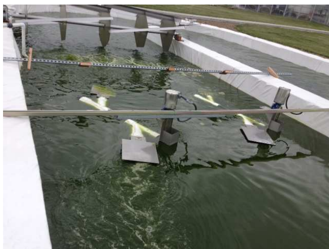
Figure 46. Redesigned water movers in operation
