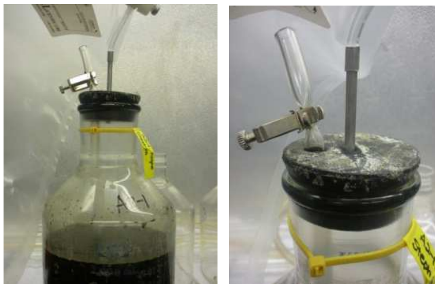
Figure 9. AD reactor modification for semi-continuous feeding of algal sludge and FOG
