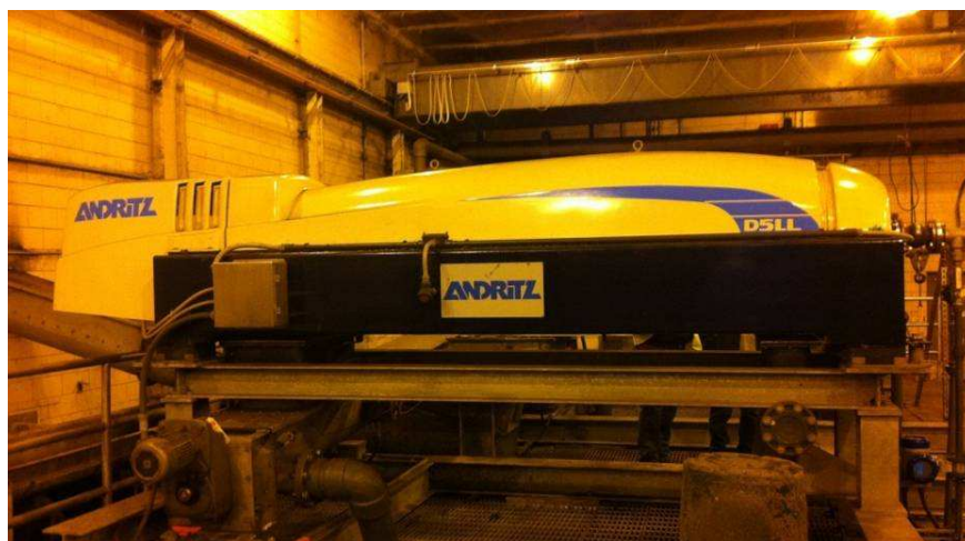
Figure 41. The ANDRITZ centrifuge system, which is used to prepare the AD effluent for algae cultivation
