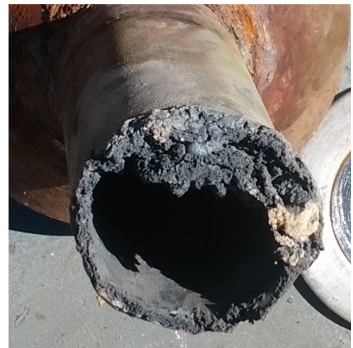
Image 12 – Damage observed on slurry feed lance (post testing)
