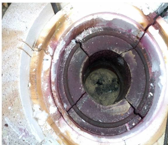
Image 8 | Combustion vessel with refractory installed (post testing)
