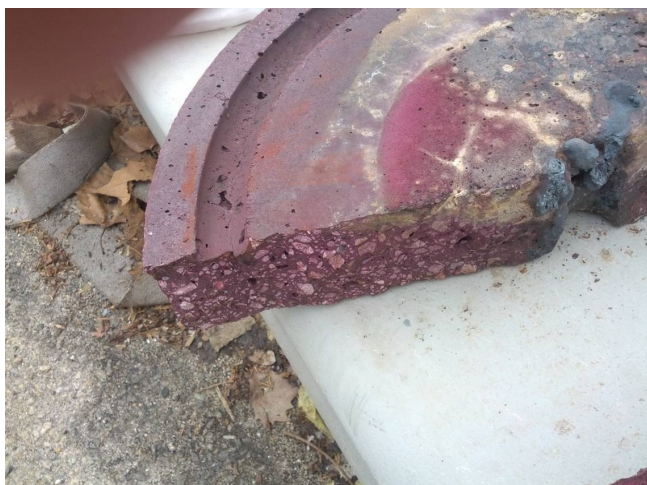
Image 14 | Close up to damage on top wall of combustion unit (post testing)
