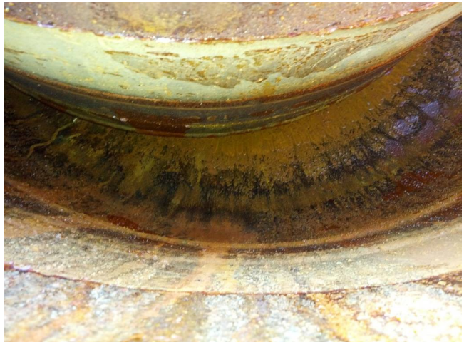
Image 10 | Gap between vessel wall and refractory (post testing)
