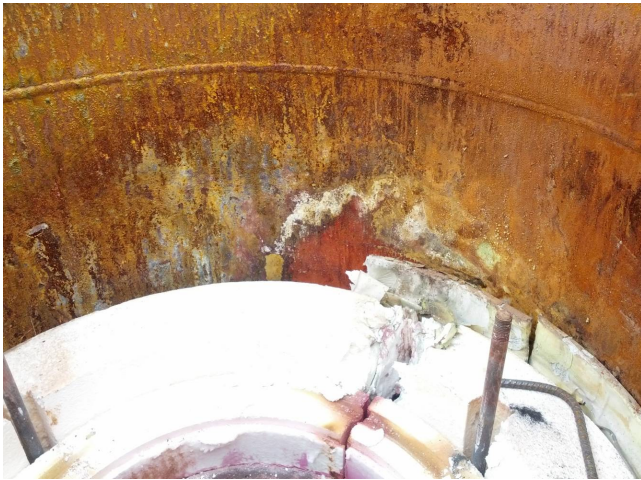
Image 9 | Condensation in vessel chamber (post testing)
