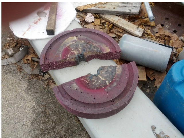
Image 13 | Top wall of combustion unit (post testing)
