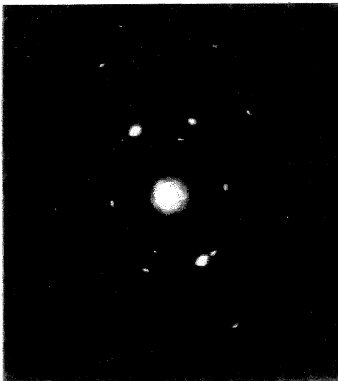
Figure 3. Typical Selected Area Diffraction with Single Crystalline Diffraction Patterns. This diffraction pattern can be identified as sodium hydroxide hydrate.
