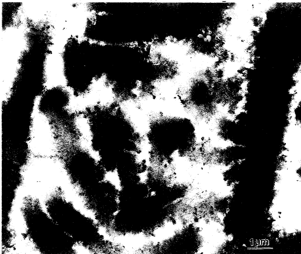
Figure 1b. TEM Image of SY-101 Sample under High Magnification. The needle-like shape and rough surface of the particles are typical of dried salts.
