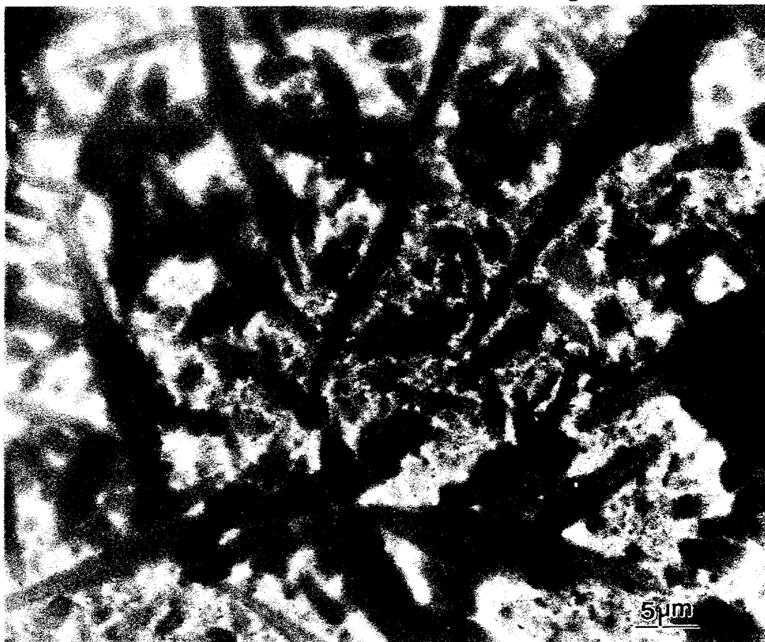
Figure 1a. TEM Image of SY-101 Sample. Needle-like particles larger than 5\mu\text{m} are observed.
