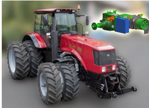
Figure 11. Belarus 3023 tractor with electro-mechanical powertrain. 27
