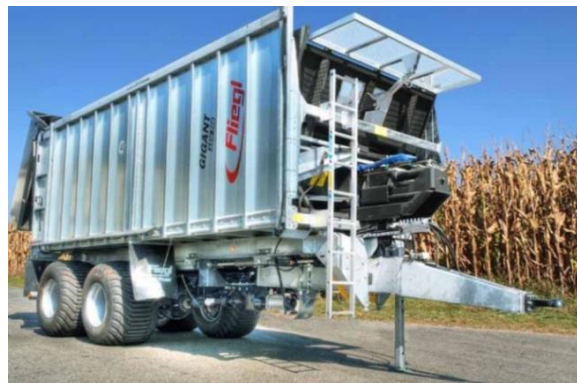
Figure 18. Trailer with electrically powered traction axle. 57
