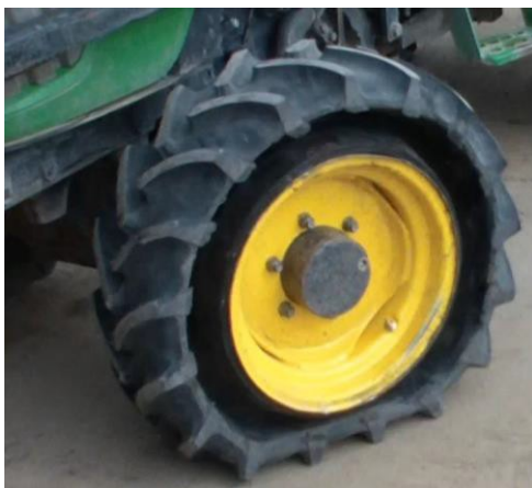
Figure 22. Galileo wheel with accordion-shape sidewall design. 78
