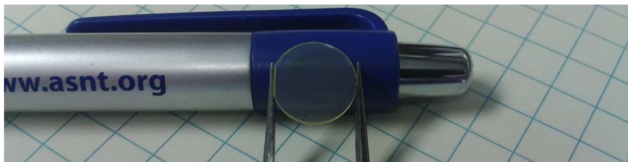
Figure 3-8. ZnO piezoelectric crystal prior to incorporation into transducer.
