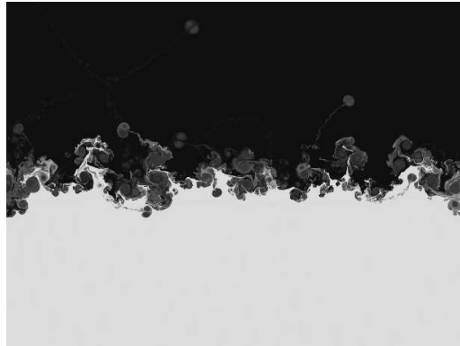
Figure 1: Contour flood of volume fraction for an At^+ = 0.5 simulation of the two-dimensional Richtmyer-Meshkov instability at a grid resolution of 4096 \times 4096 .
