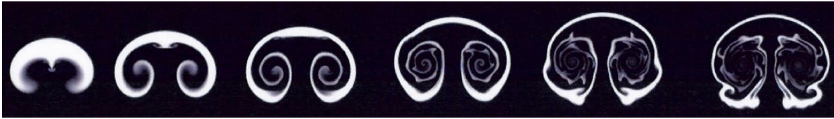
Figure 1: Contours of heavy gas mass fraction obtained with LES. Time increasing from left to right.
