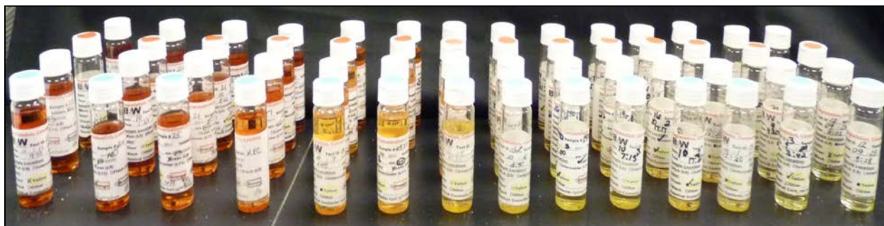
Figure 45. Solvent Color Changes during the OptiCap Solvent Testing.
