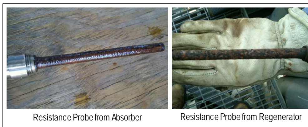
Figure 43. Electrical Resistance Probes Inspected during OptiCap Solvent Testing.
