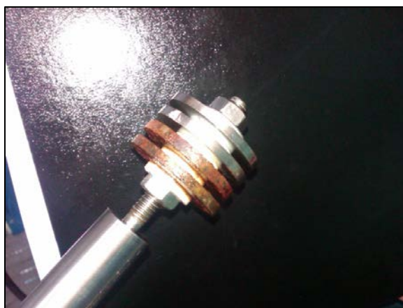
Figure 44. Weight Loss Coupons on Retractable Holder Inspected during OptiCap Solvent Testing.
