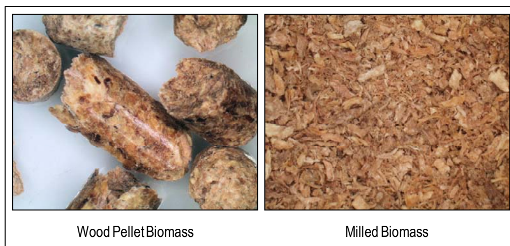
Figure 43. Wood Pellet Biomass Used as Gasification Feedstock in R03 and R04.
