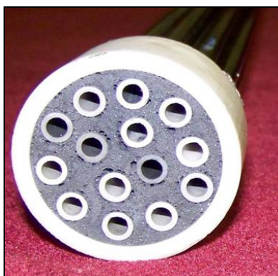
Figure 31. Media & Process Technology Hydrogen Membrane Assembly.
