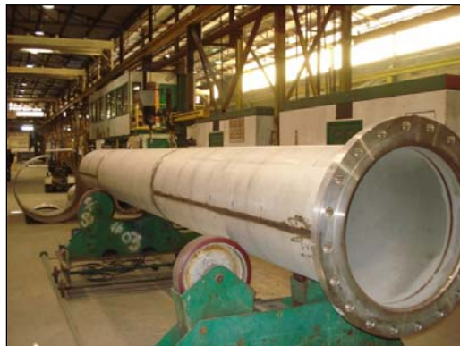
Figure 15. Fabrication of PSTU Columns.
