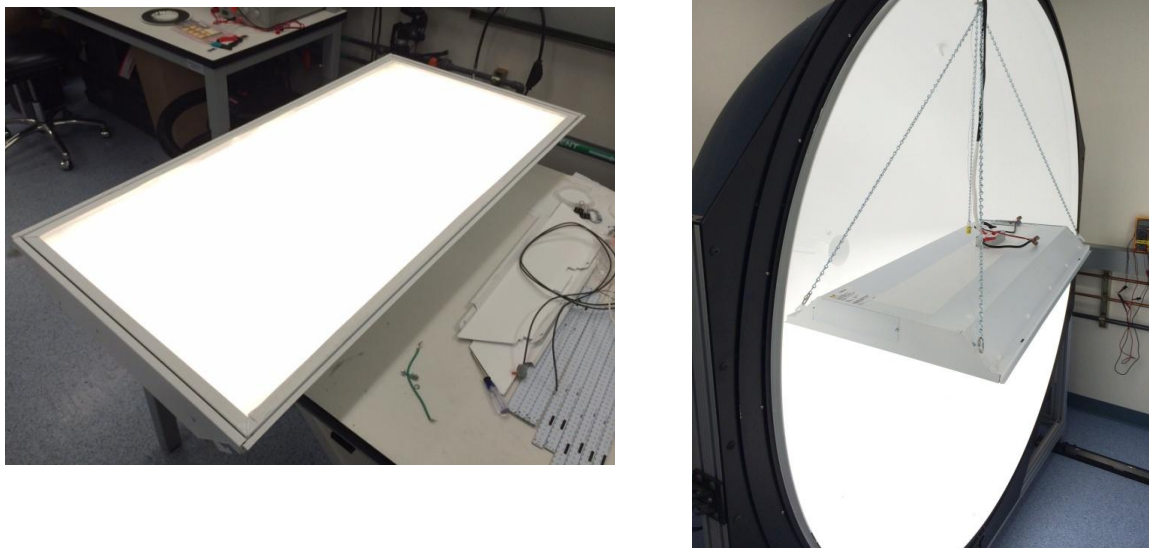
Fig. 46. Left: Demonstration troffer with diffuser in place. Right: Troffer mounted in integrating sphere for performance evaluation.
