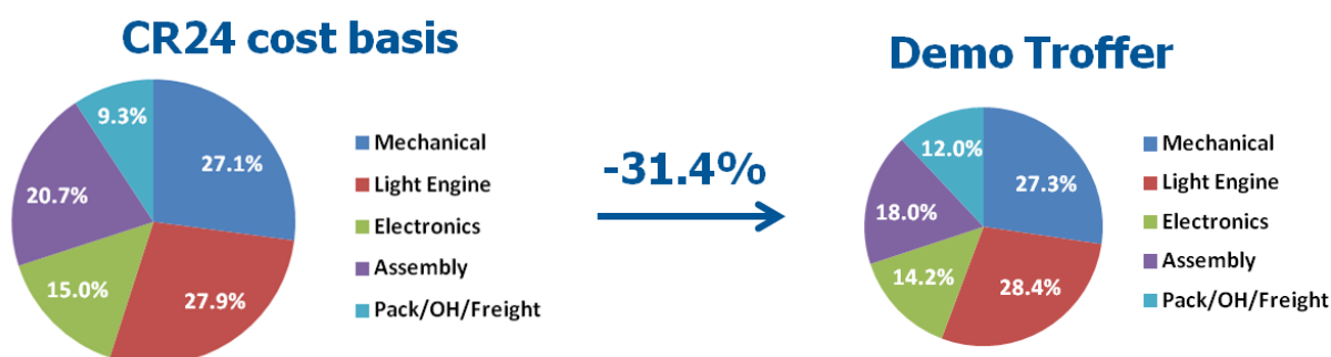
Fig. 48. Cost reductions enabled by the demonstration luminaire architecture relative to Cree's CR24 luminaire at program start. Pie chart areas are scaled by total cost.
