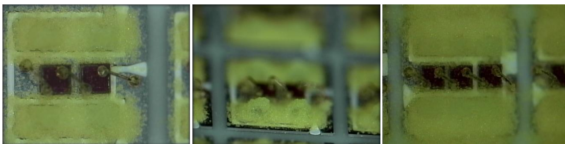
Fig. 30. Micrographs of challenges encountered during initial trials of selective phosphor application. Left: overlap with red chip positions; center: pile-up of phosphor on blue chips; right: phosphor buildup on red chip wire bonds.
