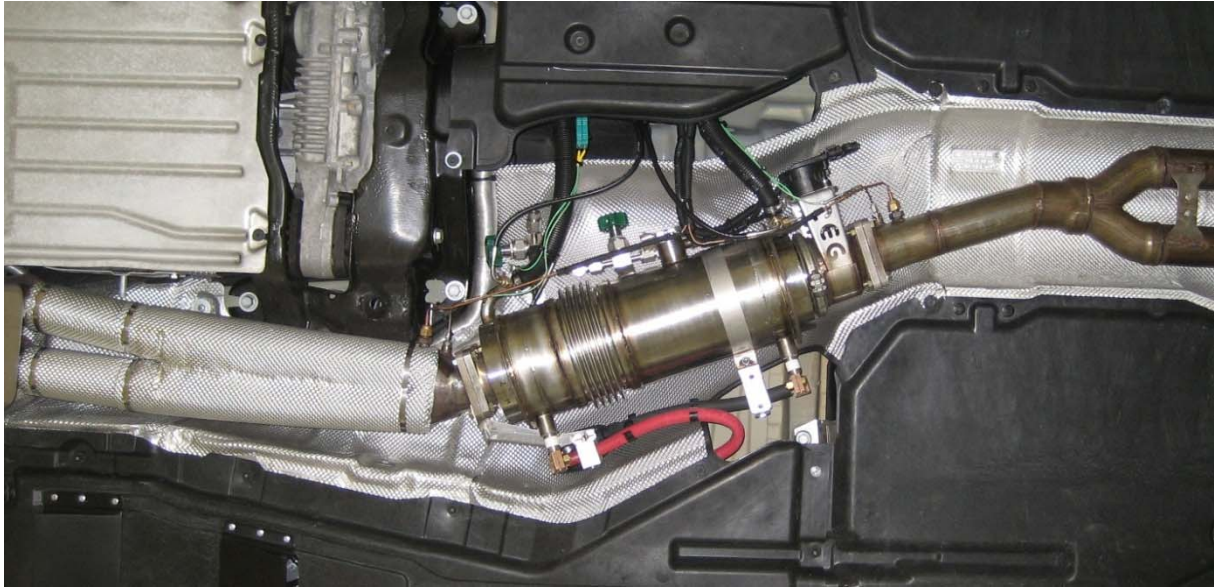
Figure 47: TEG integration into the exhaust line of the BMW X6 prototype vehicle
