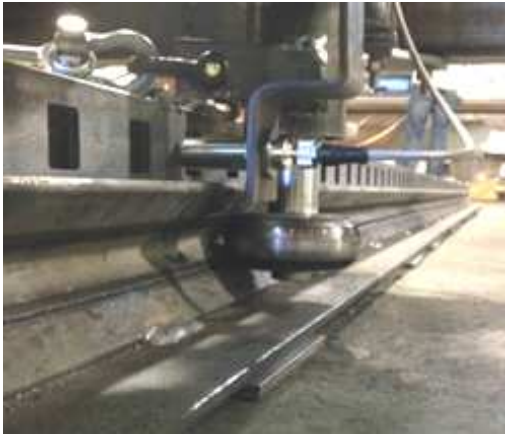
Figure 11 Testing of azimuth track friction drive showing proximity sensor and laser-cut encoder
