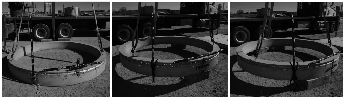
Figure 8 Photogrammetric evaluation of concrete ring and track deflection as a function of support condition
