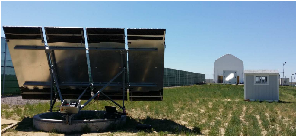
Figure 16 ROP tracking the sun on to the beam characterization target
