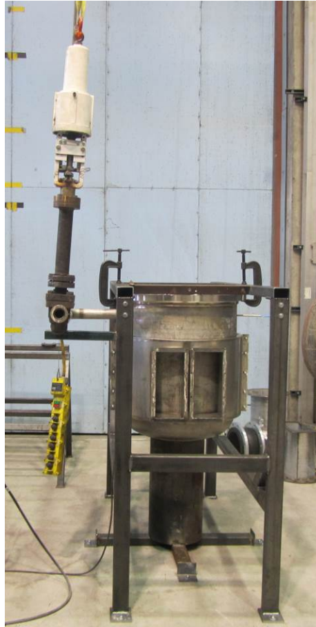
Figure 7: The Tank Positioned in the Assembly Stand, with Flow Control Valve and Cooling Ductwork Attached.
