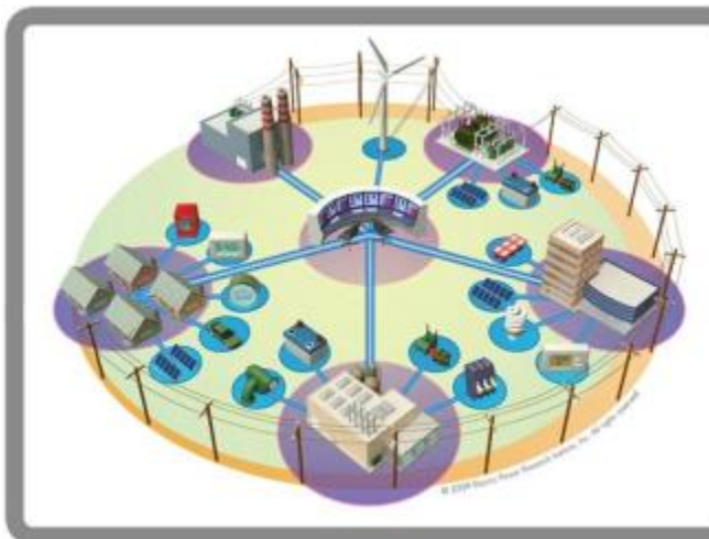
Figure 4 - Virtual Power Plant Aggregation
