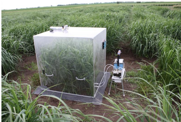
Figure 1. Plexiglass chamber for labeling field-grown switchgrass plants.
