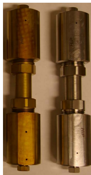
(b) Acid/heat treated vessel (left) and untreated vessel (right)
