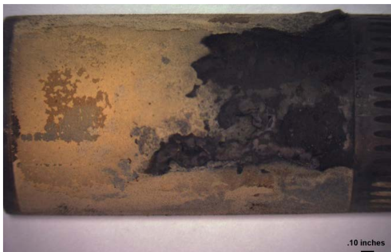
Figure 67 - Photo of the Black Thunder PRB Sleeve from the Reducing Zone, Top, Position #3.
