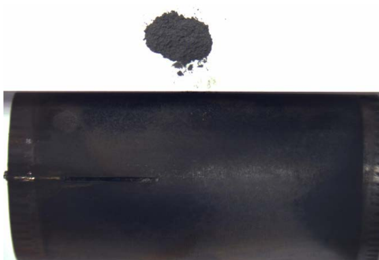
Figure 71 - Photo of the Beulah Zap Lignite Sleeve from the Reducing Zone, Top, Position #4.
