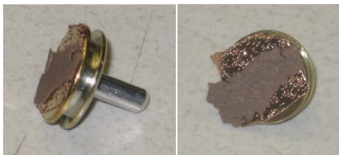
Figure 235 - Photographs of Oxidizing Deposit Flake Mounted on Stubs for SEM/EDS Analyses.
