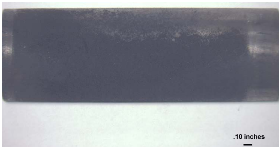
Figure 92 - Photo of Pittsburgh #8 Coal from Reducing Zone, Top Position #3.
