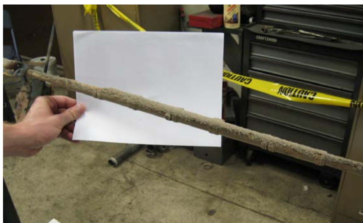
Figure 50– Air-Cooled Deposition Probe Removed from the Oxidizing Zone of Illinois #6-1 Test.
