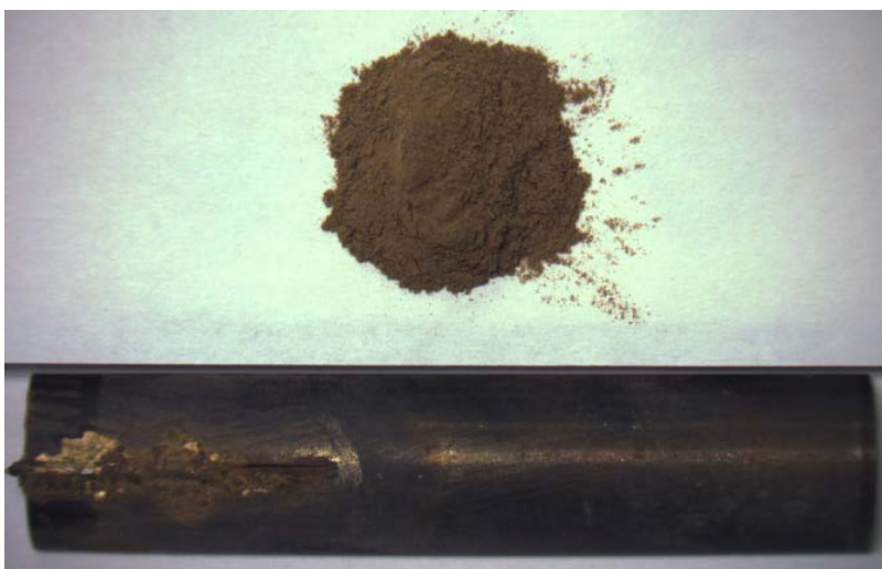
Figure 70 - Photo of the Beulah Zap Lignite Sleeve from the Oxidizing Zone, Top, Position #4.
