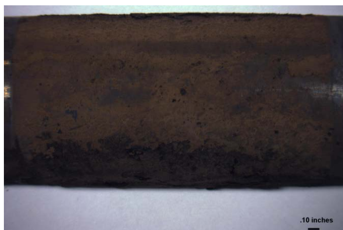
Figure 63 - Photo of the Illinois #6 Galatia Sleeve from the Reducing Zone, Bottom, Position #4.
