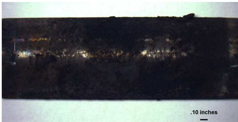
Figure 88 - Photo of KY #11 Coal Sleeve from Reducing Zone, Bottom Position #3.
