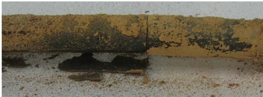
Figure 234 - Photograph of Oxidizing Deposit Probe After 450 Hours of Testing in the HMFR.
