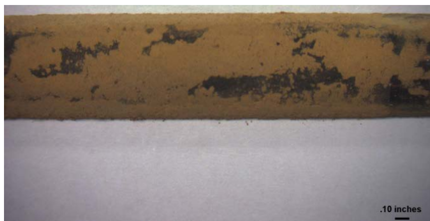
Figure 66 - Photo of the Black Thunder PRB Sleeve from the Oxidizing Zone, Top, Position #3.
