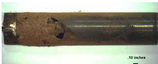
Figure 83 - Photo of OH Gatling Coal Sleeve from Oxidizing Zone, Top Position #4.
