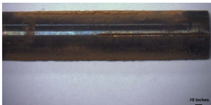
Figure 60 - Photo of the Illinois #6 Galatia Sleeve from Oxidizing Zone, Top, Position #4.
