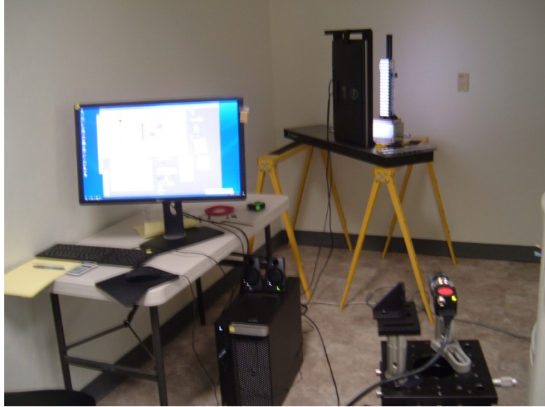
Fig. 13 Overall test SRD set up for Si plane mirror
