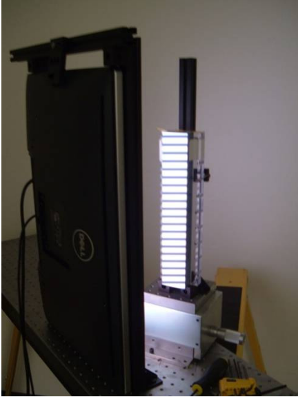
Fig. 12 Fringes reflected off 300mm x 50mm Silicon plane mirror
