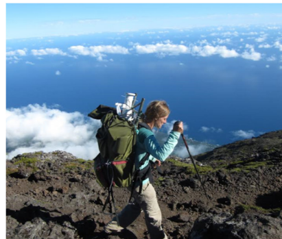
Figure 17: Graduate student Kendra Wright hiking to PMO and carrying the instrumented cargo backpack. The white cylinder protruding from the top of the backpack is part of the cell of the nephelometer.
