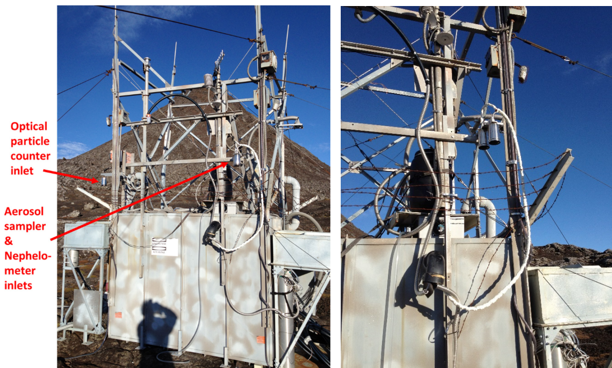
Figure 5. Optical particle counter, aerosol sampler and nephelometer inlets (left) and a zoomed in picture of the heated sampler and nephelometer inlets installed at the station during year 1 of this project (summer of 2012).
