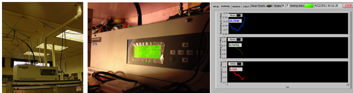
Figure 3. The set-up for the Aurora 3000 nephelometer in the Environmental Optics Laboratory at MTU during the calibration/test sessions in March of 2012 (left panel). The nephelometer installed inside the PMO in summer of 2012 (middle panel). Right panel: custom-made Lab-View code developed for acquiring the scattering, backscattering, temperatures, RH and pressure data from the Aurora 3000. The software collects data every 10 seconds and calculates 10-second averages and standard deviations for plotting and data archival. The solid lines represent 10-second averages, while the dashed lines represent the standard deviations. The blue line represents data (in inverse megameters) collected at 450 nm, the green at 525 nm and the red at 635 nm.
