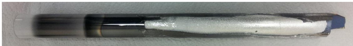
Figure 6. Shows the further purified Mg after resublimation of the material obtained in the first run. This time the left over, unsublimed residue is almost negligible.
