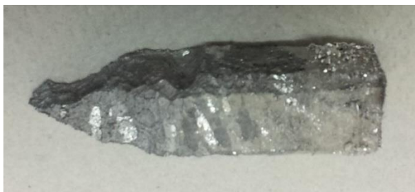
Figure 5. The sublimed Mg of improved purity. Shows a typical residue found in the crucible and the remaining part of the original (solid) starting material.
