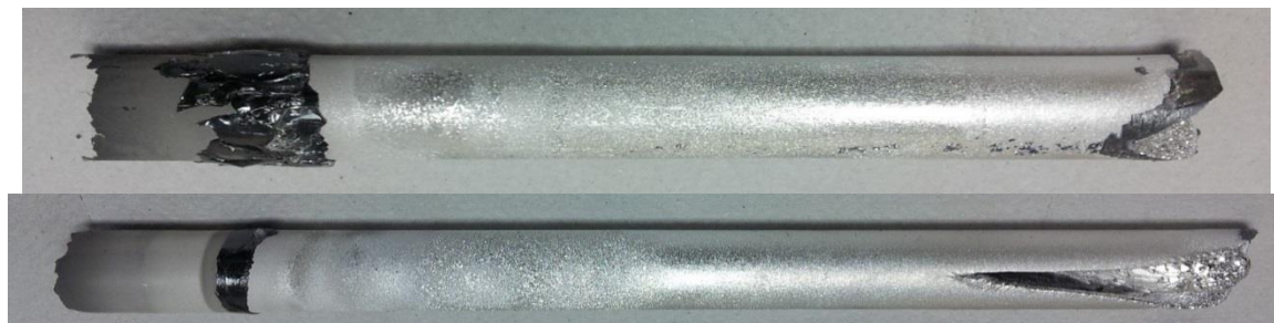
Figure 7. At the outer end of the deposit, where the magnesium deposits on the cold end of the tubing, there was a 2-3 cm strip where silica sticks very strongly to the metal.
