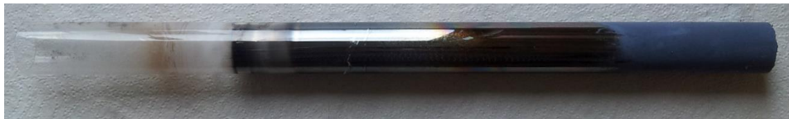
Figure 4. After sublimation was complete, the pBN crucible was removed carefully from the ampoule and the sublimed and unsublimed parts were removed
