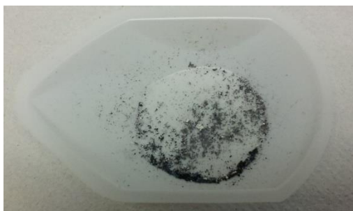
Figure 5. The sublimed Mg of improved purity. Shows a typical residue found in the crucible and the remaining part of the original (solid) starting material.
