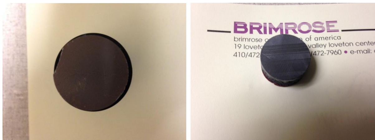
Figure 9. Left Photograph shows lapped cross section of 25 mm diameter Indium doped CdMgTe crystal and the right photograph is that of 19 mm diameter crystal. Left sample is practically twin- free.
