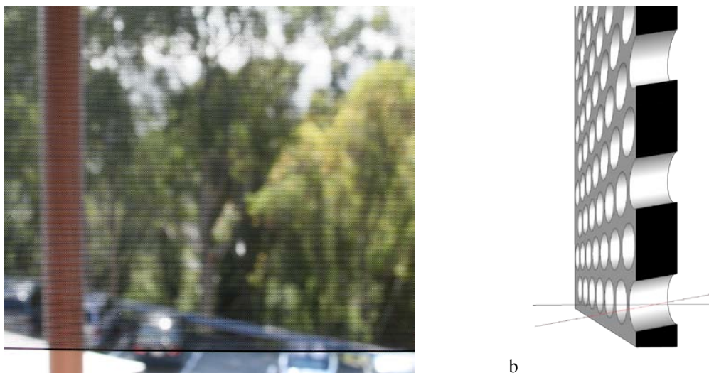
Fig. 8. (a) View through the micro-perforated shade held at arm's length and (b) a section view of the micro-perforated shade - not to scale.
