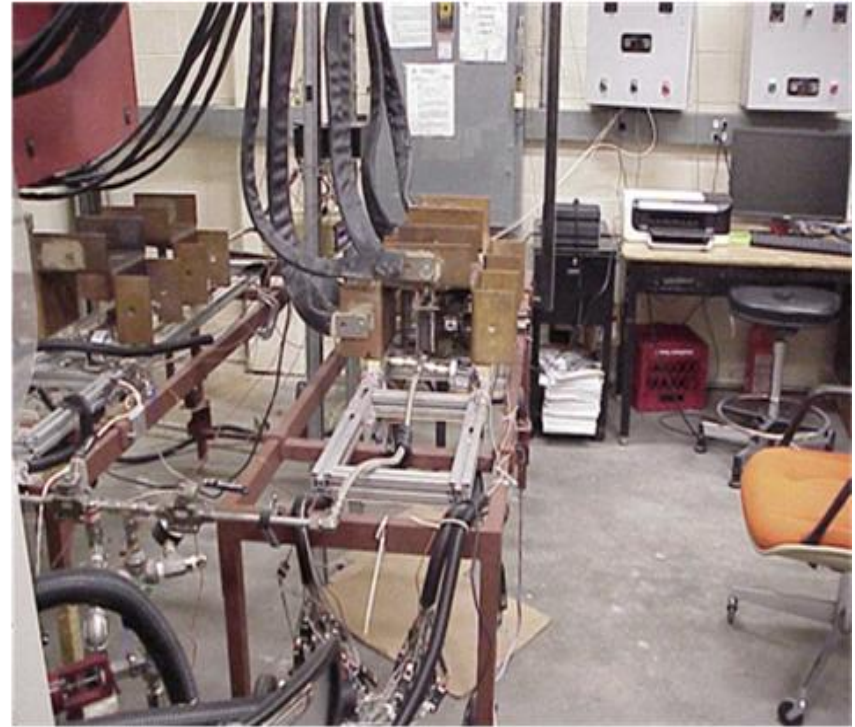
SIDE VIEW OF TEST CENTER WITH BUS CABLES, TEST SECTION, ALUMINUM NITRIDE, FLUID FLOW, HEATER & MYKROY
