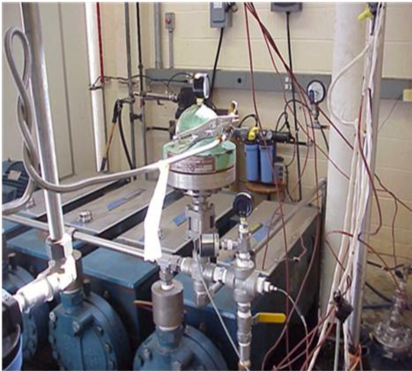
FRONT VIEW OF PRESSURE TRANSDUCER WITH THERMOCOUPLE, FLOW LOOP PUMPS, AND PRESSURE STABILIZER
