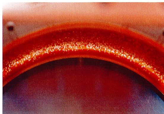
Figure 2: Breakdown damage on the iris of an 805 MHz pillbox cavity, after high-power testing in a magnetic field ramped from 0 to 3 T. ~1 mm-diameter damage spots are distributed around the entire circumference of both cavity irises, as well as the end walls and opposite the input coupler (not shown). Photo credit: Fermilab Visual Media Services.
