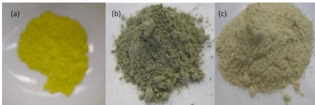
Figure 2.2.11. Appearance of the \text{BiVO}_4 (a), \text{Bi}_2\text{WO}_6 (b) and \text{AgBiW}_2\text{O}_8 (c) samples prepared by SCS and using urea as fuel.
