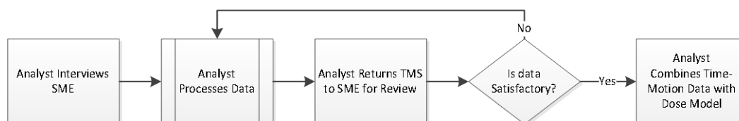
Figure 14. Example flow sheet for the development of a time-motion study for operations currently in practice
