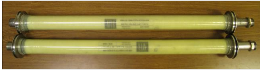
Figure 34. MTR's Hydrogen Membrane Modules Tested in R12
