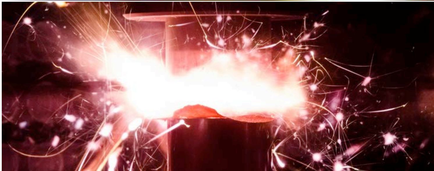
Comprehensive energetic materials development, characterization, and testing are strengths at Los Alamos National Laboratory. An experimental explosive is shown igniting during small-scale impact testing.
