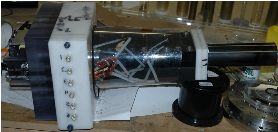
Figure 64 HyperV plasma railguns are three stage linear plasma accelerators. First Neutral gas is injected with an electromechanical fast gas valve (GV). Next the pre-ionization stage (PI) ionizes the gas electrothermally using a capillary discharge channel. This injects a plasma armature into the final railgun acceleration stage. Here the plasma armature is accelerated via a Lorentz force, generated by current from a Pulse Forming Network (PFN), and ejected as a high velocity plasma jet.
