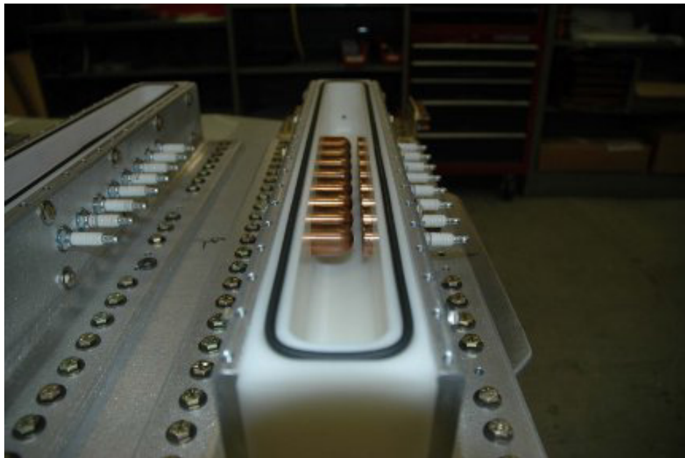
Figure 63 Closeup of the internal switch cavity showing electrodes and spark plug ignitors.
