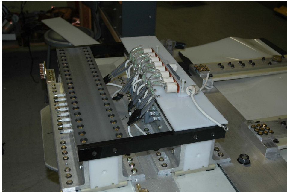
Figure 59 A 12 inch long version of early top trig linear spark gap switch.
