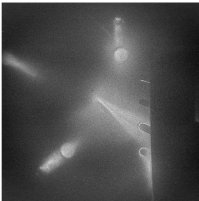
Figure 104 Imaging off axis late in time (after peak density at merge point) shows formation of a collimated jet. The pressure probe array is seen on the right side of the image. The image is taken through the same port as the spectroscopy parallel collection optics in Figure 99.
