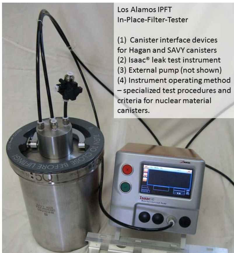
Figure 9. The Los Alamos IPFT (In-Place-Filter-Tester) system.
