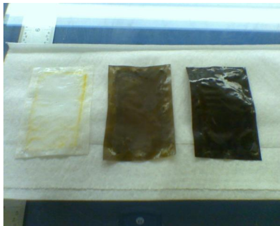
Figure 107. Separators taken from LFP-graphite cells after formation (left), 10 overcharge cycles (middle) and overcharge cycling to failure (right)
