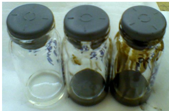
Figure 106. Electrolyte drained from the LFP-graphite cells after formation (left), 10 overcharge cycles (middle), and overcharge cycling to failure (right)
