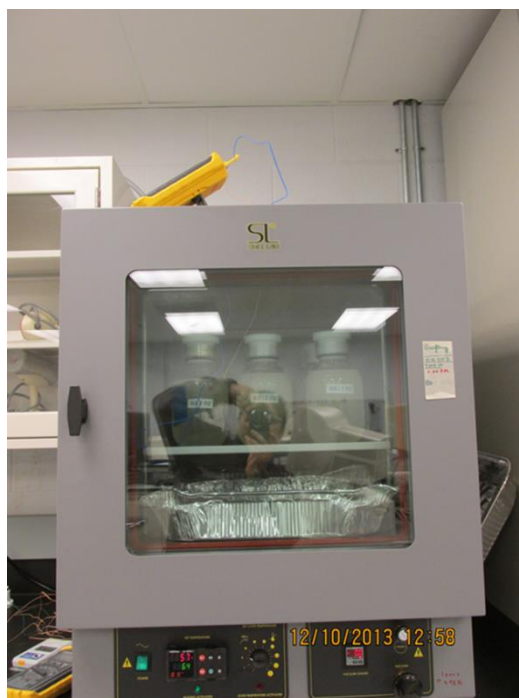
Figure 9. Glove bag containing pressure bottles and grafting solutions.
