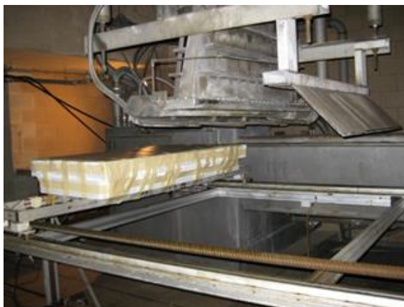
Figure 6. Electron beam set-up for irradiating adsorbent fibers.
