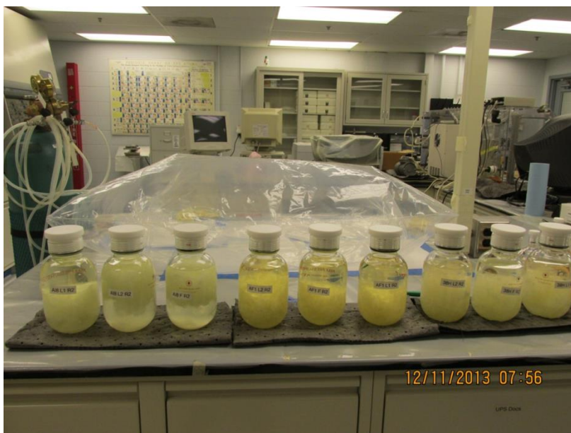
Figure 11. Adsorbent fibers after grafting reaction.
