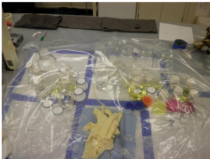
Figure 9. Glove bag containing pressure bottles and grafting solutions.
