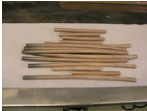
72-hour air-oxidized Zircaloy-4 tubes.
