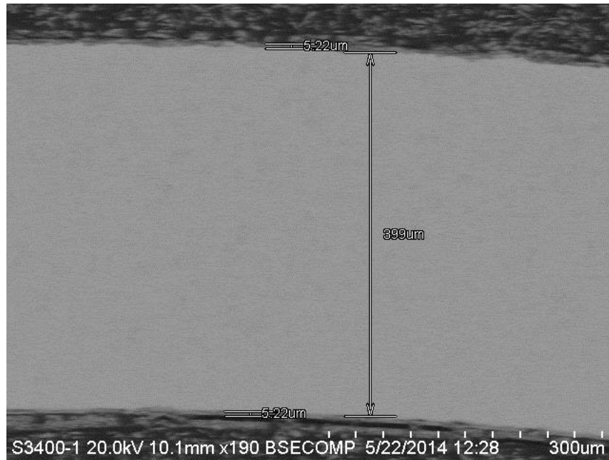
6-hour air oxidation-Zircaloy 4 tube
