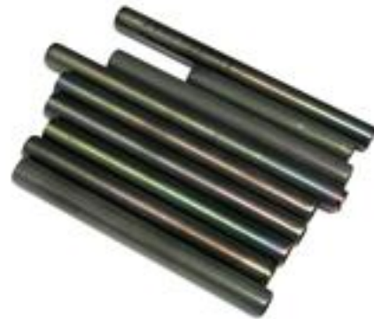
72-hour air-oxidized Zircaloy-4 tubes.
