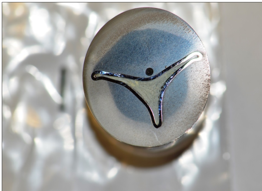
Fig. A-5. Cross section of sample 2-6 (700°C, 300 MPa).
