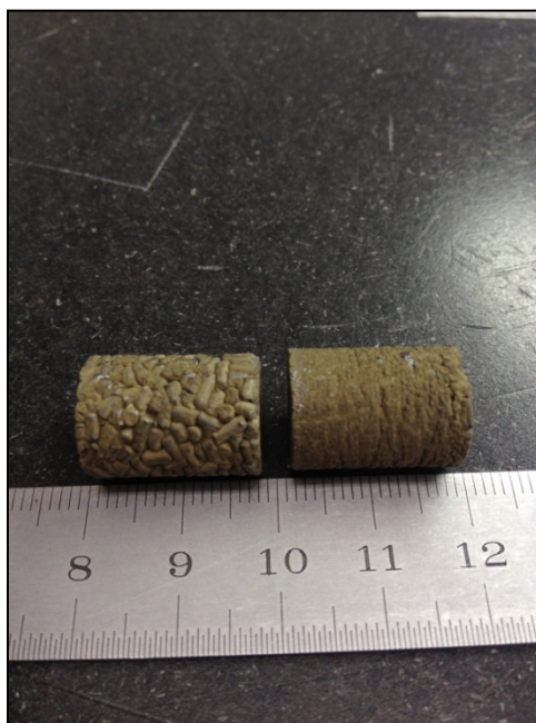
Fig. 4. Side view of HUPed compacts formed from pelletized (l) and crushed (r) engineered \text{Ag}^0\text{Z} .
