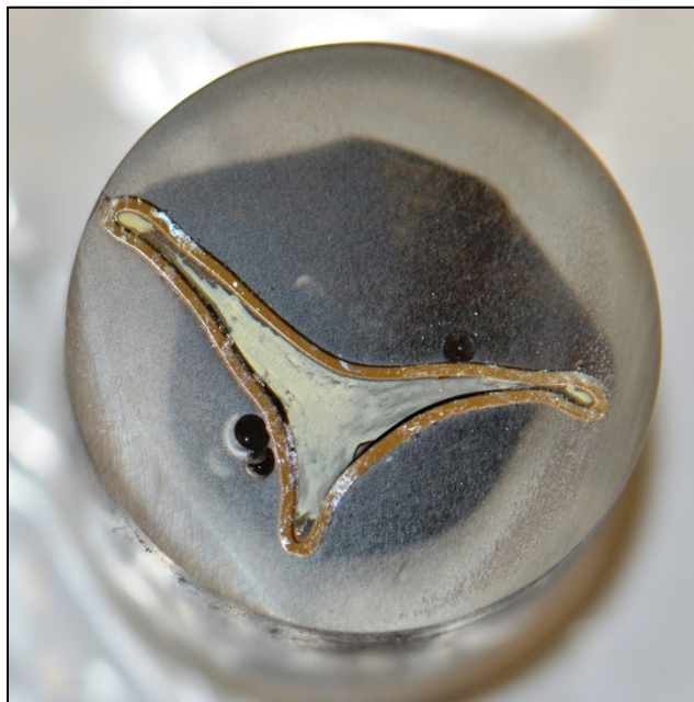
Fig. 27. Cross section of sample 2-7 (NaZ + AgI 3:1; 700°C and 300 MPa).
