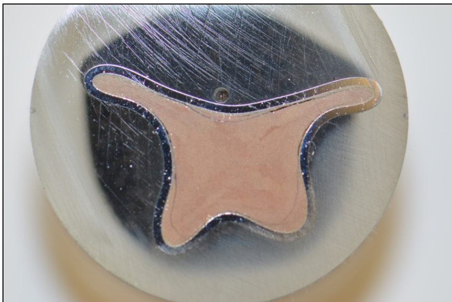
Fig. A-1. Cross section of sample 1-5 (850°C, 100 MPa).
