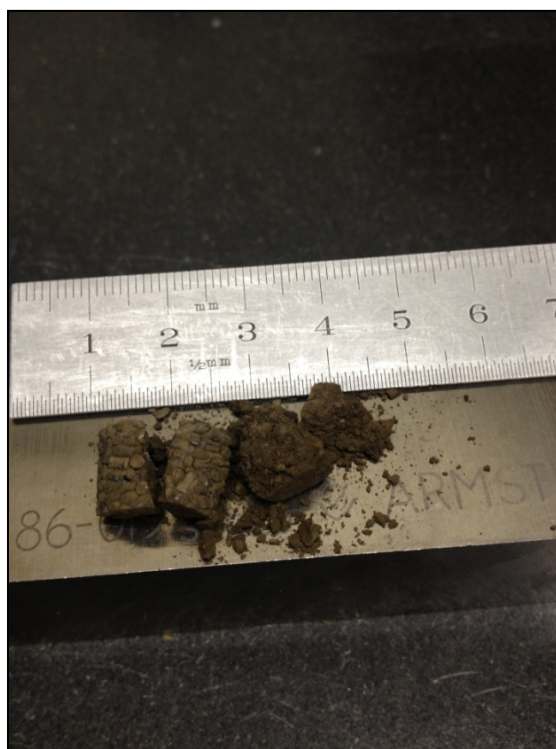
Fig. 6. Crushed HUPed compact formed from engineered \text{Ag}^0\text{Z} .
