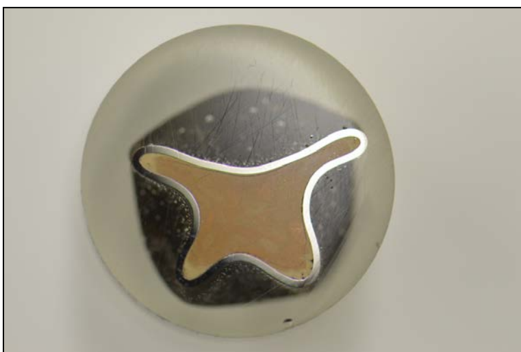
Fig. 13. Cross section of HIPed sample 1-3 (700°C and 175 MPa).
