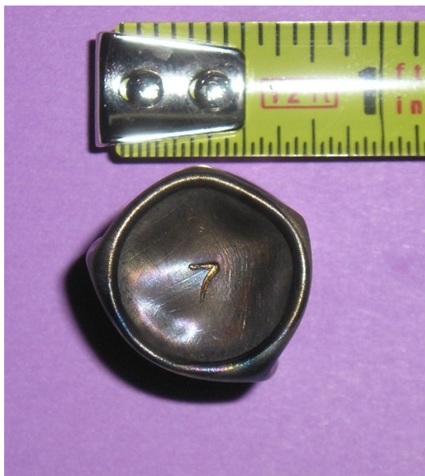
Fig. 10. HIPed capsule 1-8 containing I-Ag 0 Z.
