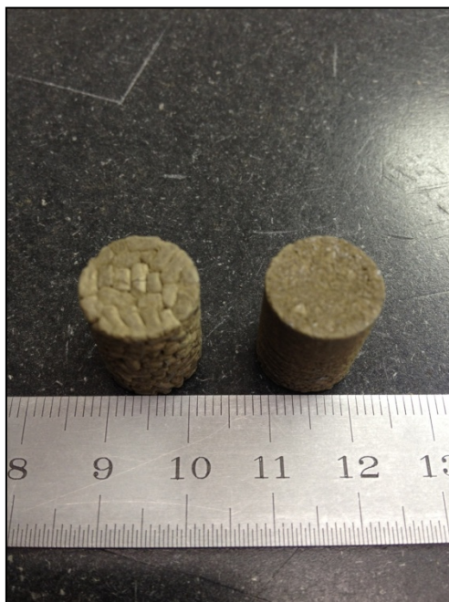
Fig. 3. HUPed compacts formed from pelletized (l) and crushed (r) engineered \text{Ag}^0\text{Z} .
