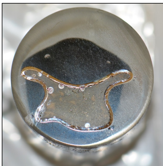
Fig. 26. Cross section of sample 2-13 (engineered Ag 0 Z + AgI 3:1; 900°C and 100 MPa).
