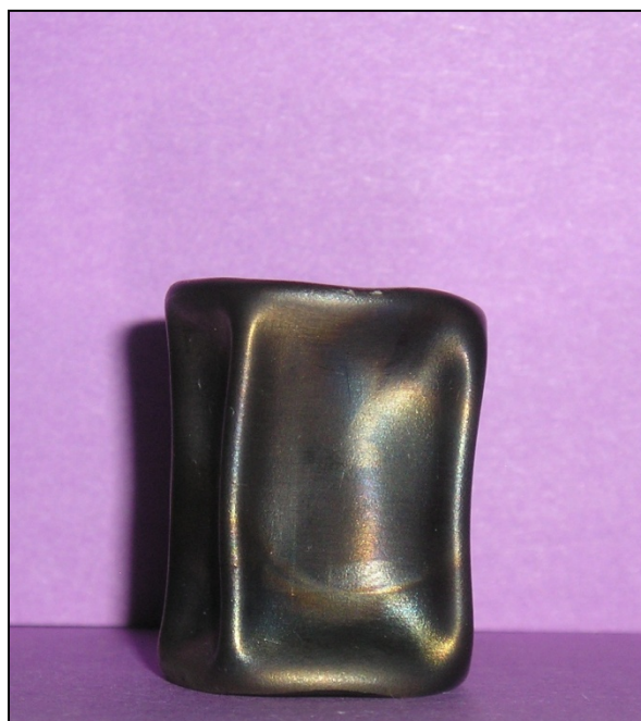
Fig. 9. HIPed capsule 1-8 containing I-Ag 0 Z.
