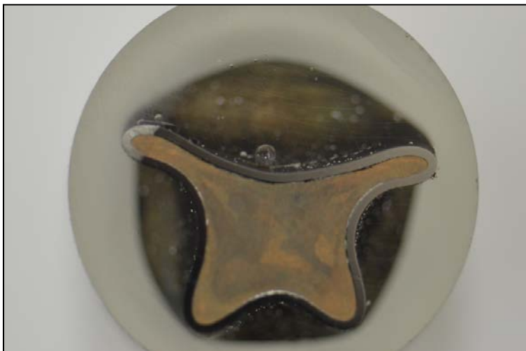
Fig. 15. Cross section of HIPed sample 1-8 containing I-Ag 0 Z (700°C and 175 MPa).
