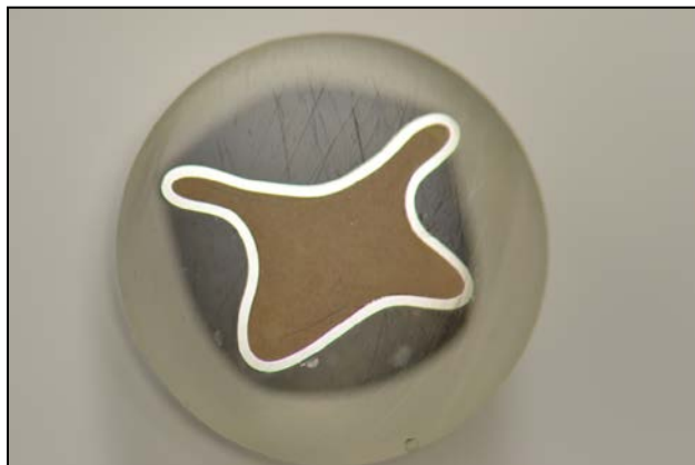
Fig. 12. Cross section of HIPed sample 1-2 (700°C and 100 MPa).
