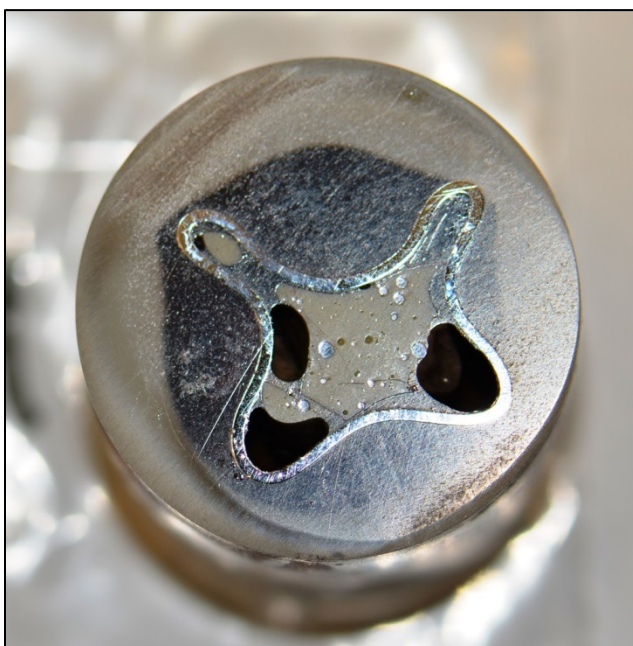
Fig. 28. Cross section of sample 2-11 (NaZ + AgI 3:1; 900°C and 100 MPa).
