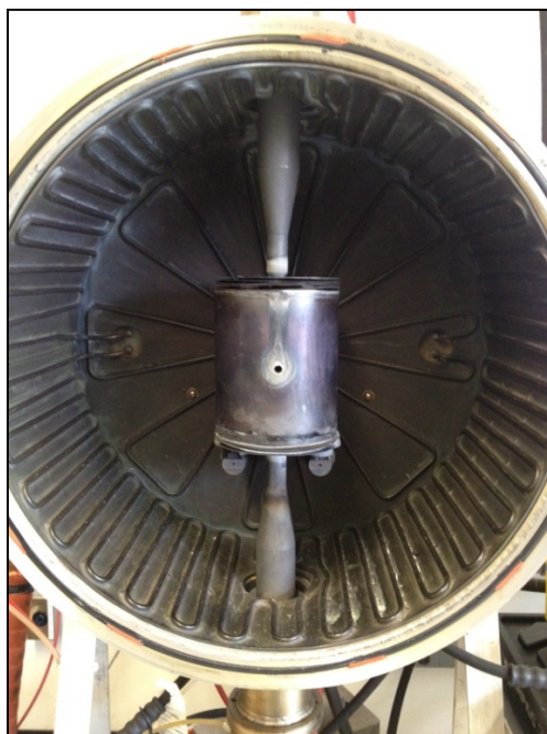
Fig. 2. Hot uniaxial press and furnace used in initial testing for \text{Ag}^0\text{Z} pressing.
