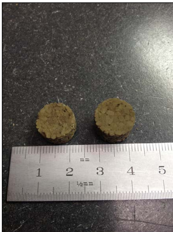
Fig. 5. Cross section of HUPed compact formed from engineered \text{Ag}^0\text{Z} .
