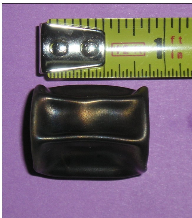
Fig. 11. HIPed capsule 1-7 containing I-Ag 0 Z.
