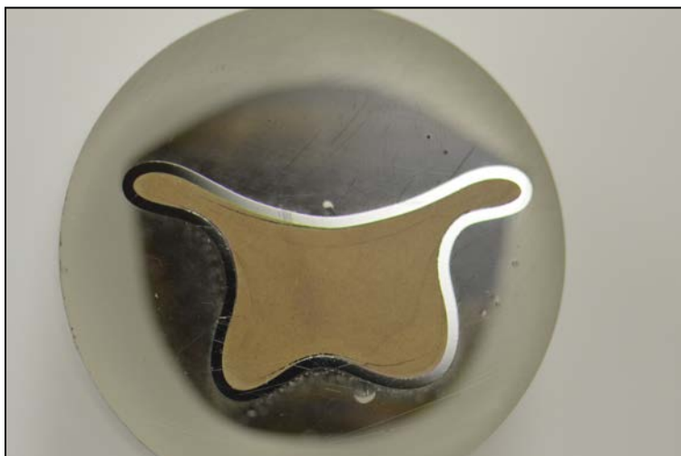
Fig. 14. Cross section of HIPed sample 1-6 (crushed Ag 0 Z, 700°C and 100 MPa).
