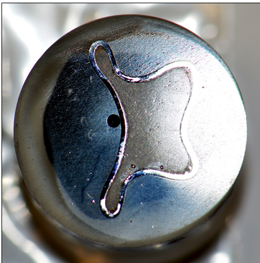
Fig. A-6. Cross section of sample 2-13 (900°C, 175 MPa).
