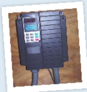
Integrated phase converter variable speed drives are available for single phase applications.
