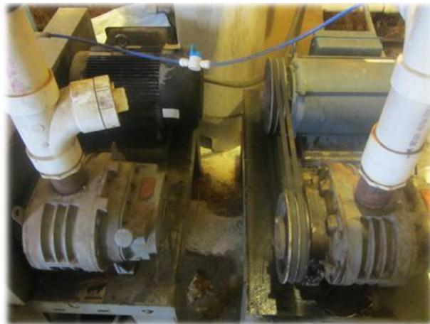
Figure 9: Lenz dairy's 10 HP and 7.5 HP vacuum pumps which operate during milking and
