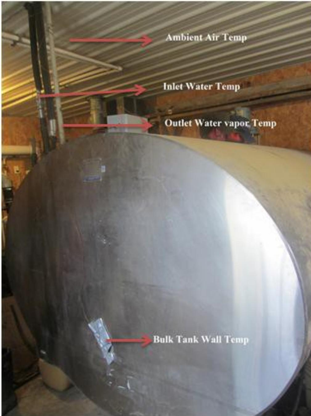
Fig. 15 The position of temperature sensors
