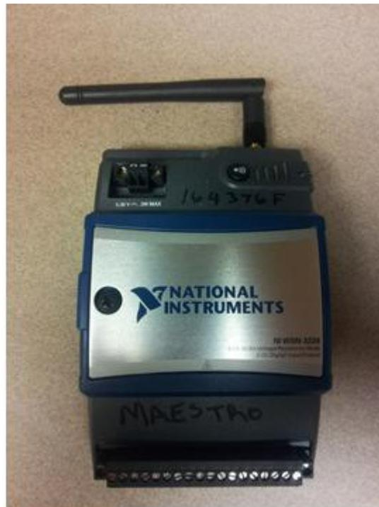
Figure 3 NI WSN-3226 Voltage/RTD combination node
