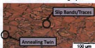
Cold-rolled Cu Micrograph
