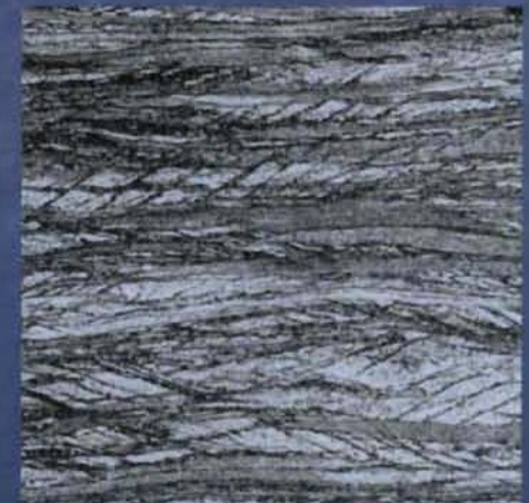
Cu Plane Strain Compression Undeformed \epsilon = -1.5
