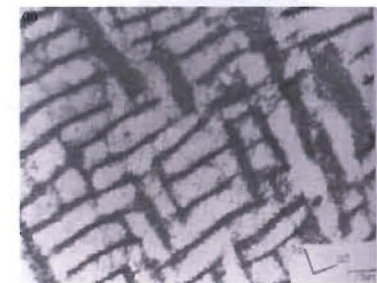
Fig. 9. Further examples of the labyrinth structure. (a) (011)-section of copper single crystal cycled in the [011] direction, Jin (1987). (b) polycrystalline Cu-Ni alloy fatigued to saturation, Charsley (1981). Reprinted by permission of Publisher.
