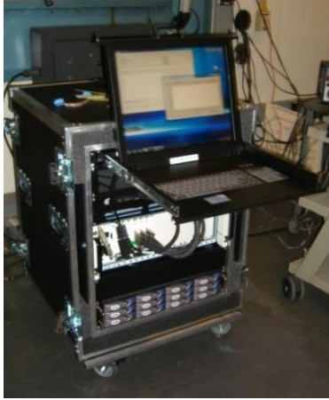
Figure 3. The BETSY list-mode data acquisition system is set up outside of the shielded cell.
