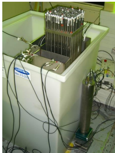
Figure 2. The original experimental setup of the DDA instrument. The 15x15 PWR fuel assembly is filled with 204 fresh LEU and DU rods. Three stainless steel enclosures hold nine ^3\text{He} detectors inserted into HDPE cylinders wrapped with Cd. The plastic tank is filled with ~76 cm of water, high enough to cover the detectors. The DT neutron generator sits directly outside of the tank, adjacent to the fourth side of the fuel assembly.
