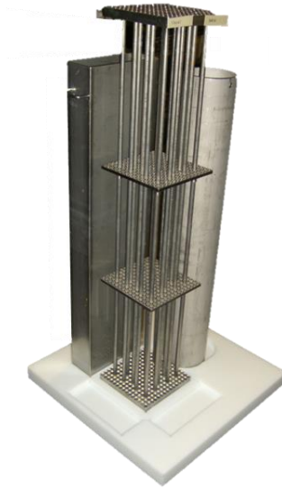
Figure 7. The updated DDA template which will hold the experimental components in fixed positions.
