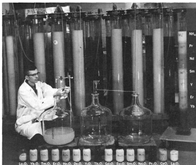
Figure 11 Ion-exchange columns used to separate the rare earths from one another. Individual rare earths are collected in the large carboys as they are removed from the columns. The jars in front of the chemist contain the oxides of the individual rare earth elements.
