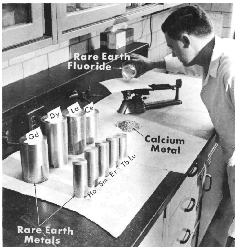
Figure 12 Some rare earth metals as prepared from their fluorides. The four samples in the back row are 10 cm in diameter, and the five in the front row are 5 cm in diameter. The chemist is weighing out a rare earth fluoride, which he will mix with the calcium chips to prepare some more rare earth metal.
