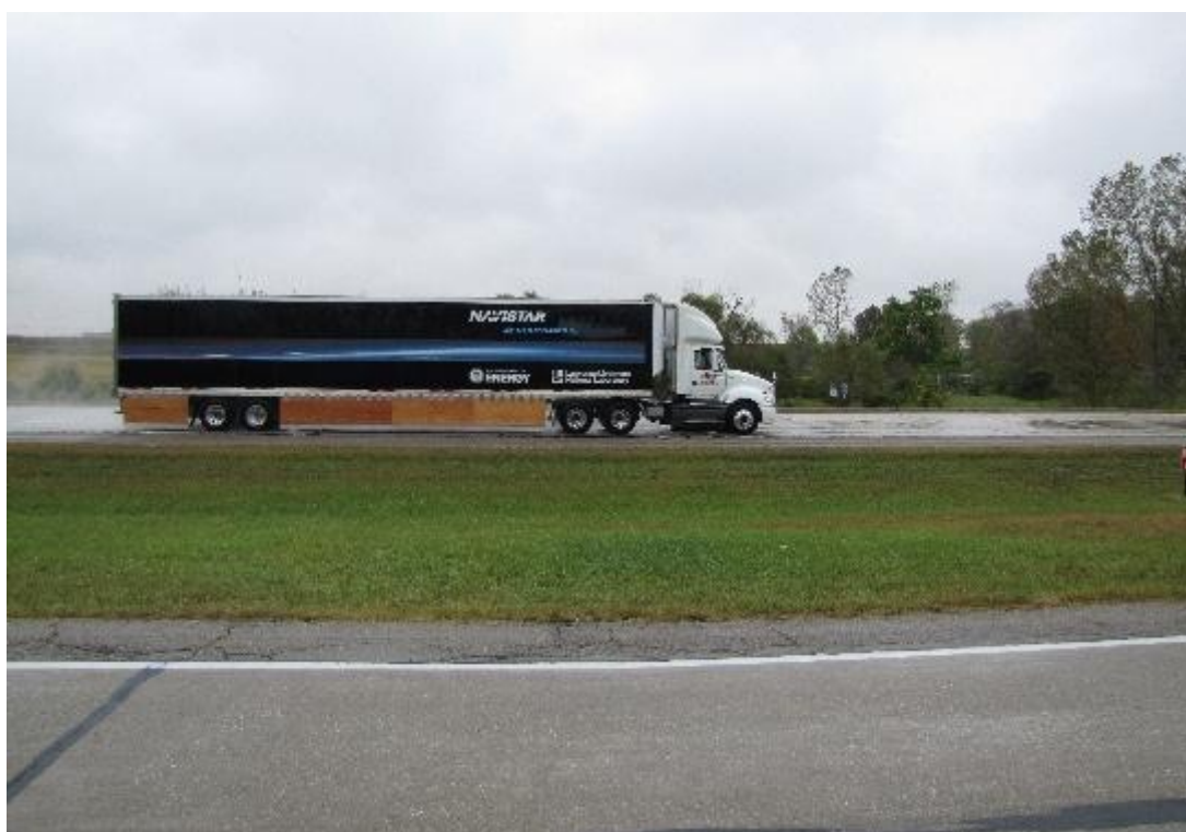
Configuration 12: Freight Wing Gap Fairing and LLNL Skirts
