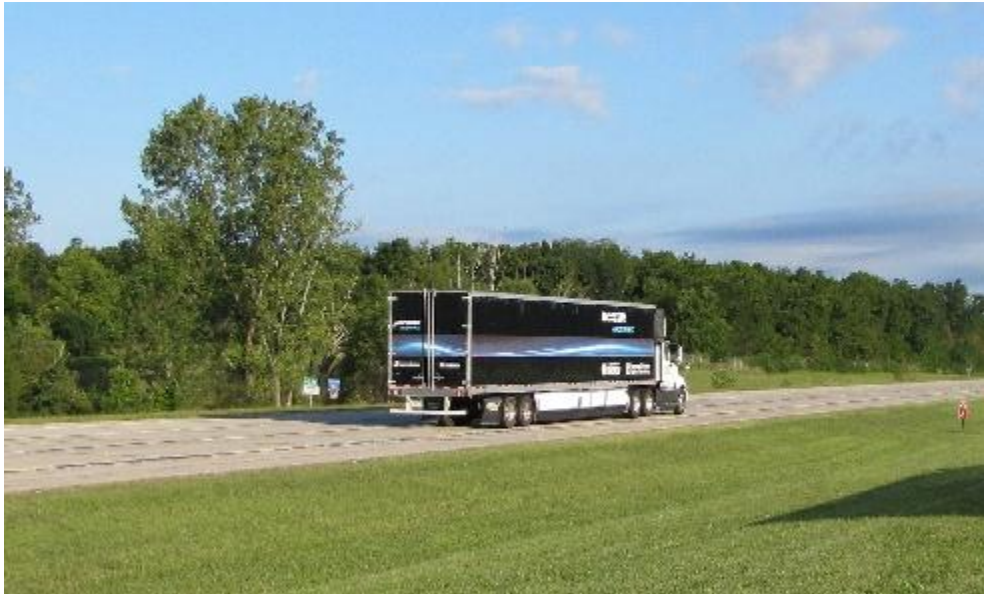
Configuration 4: Freight Wing Gap Fairing
