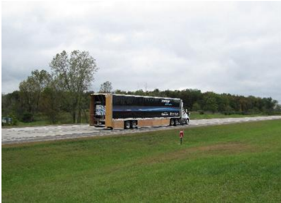
Configuration 13: Freight Wing Gap Fairing, LLNL Skirts, and LLNL 3-Sided Boat Tail
