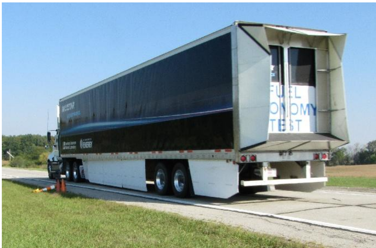
Configuration 12: Freight Wing Gap Fairing and LLNL Skirts
