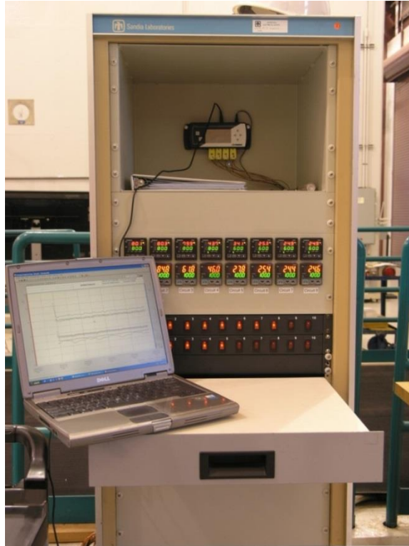
Figure 11 New controller system that was designed and built in FY14. It allows for independent control of eight heated LICA exposure cans.
