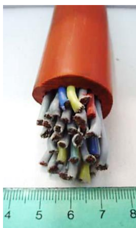
Figure 1 - Silicone rubber cable specimen (scale in centimeters); photo taken from previously published report [6].
