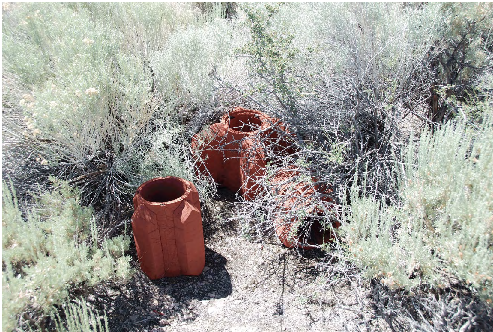
Figure 359. Feature 188, casing centering sleeves (insulators) at the U-12n.03 #1 CH, U12n Tunnel, view east (2008).
