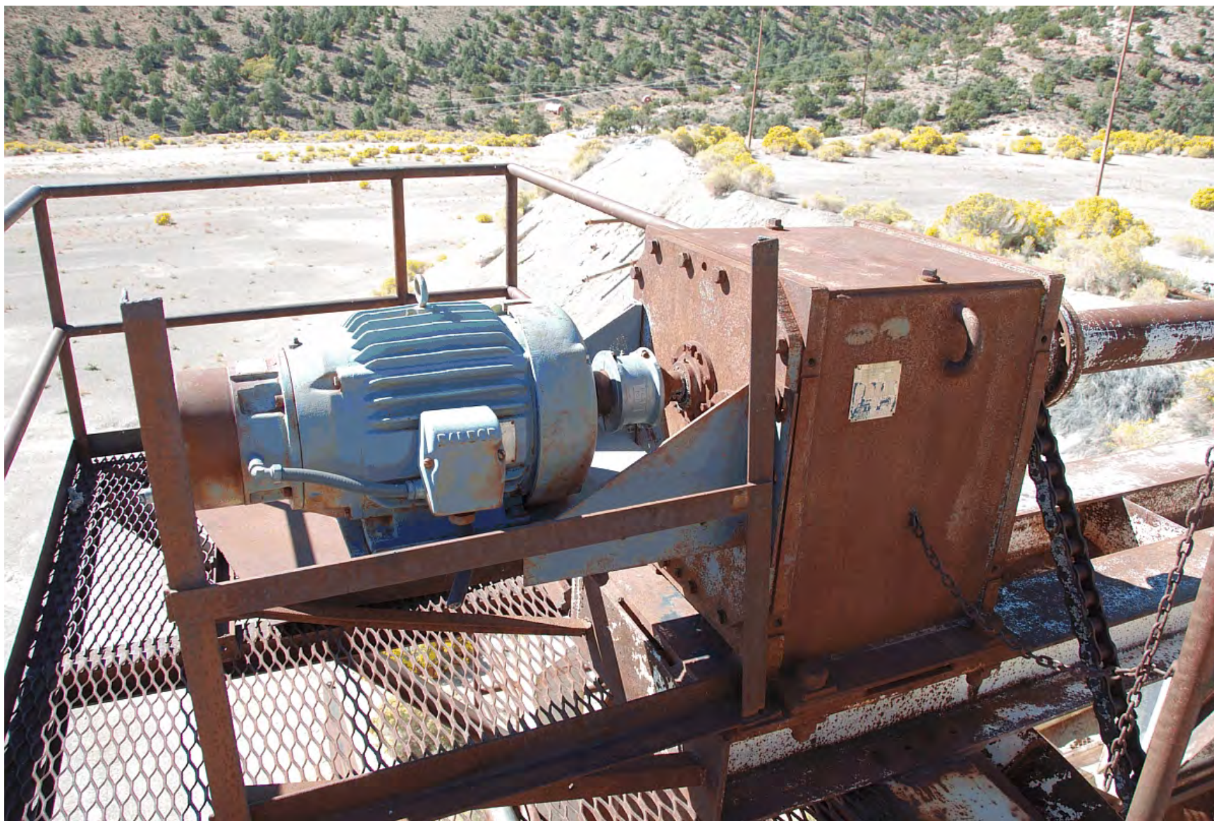
Figure 188. Feature 45, motor and gear reducer, U12n Tunnel, view south (2008).
