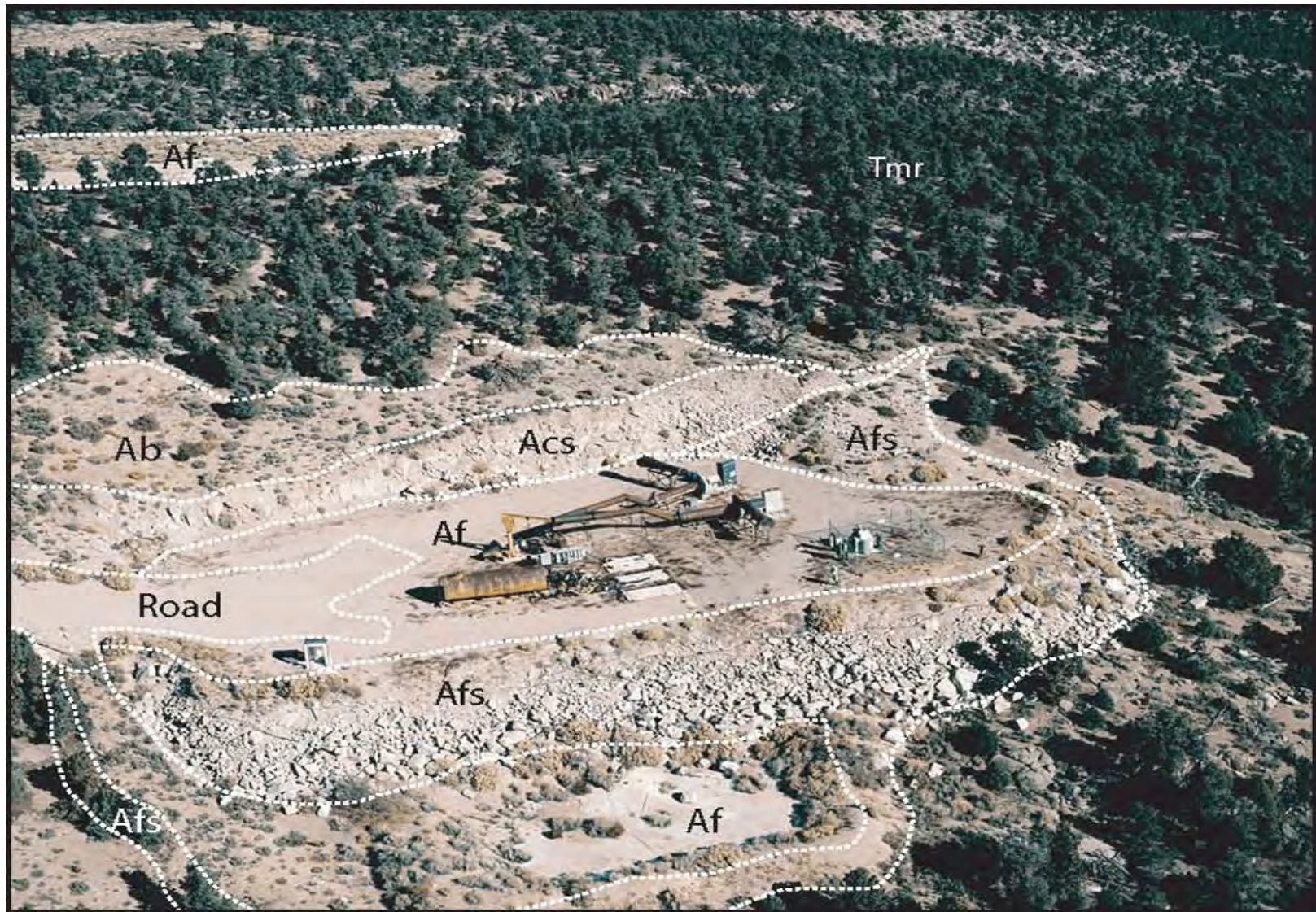
Figure 112. View of the U12n Tunnel vent hole No. 1 and chiller pad. Shown are bedrock cut slope (Acs) with bladed colluvium above the cut slope (Ab), fill pads (Af), and fill slopes (Afs). The excavated bedrock material was used in the development of the pad and facing of the fill slopes. (modified from photograph NF-13506, on file at the Remote Sensing Laboratory, Las Vegas)
