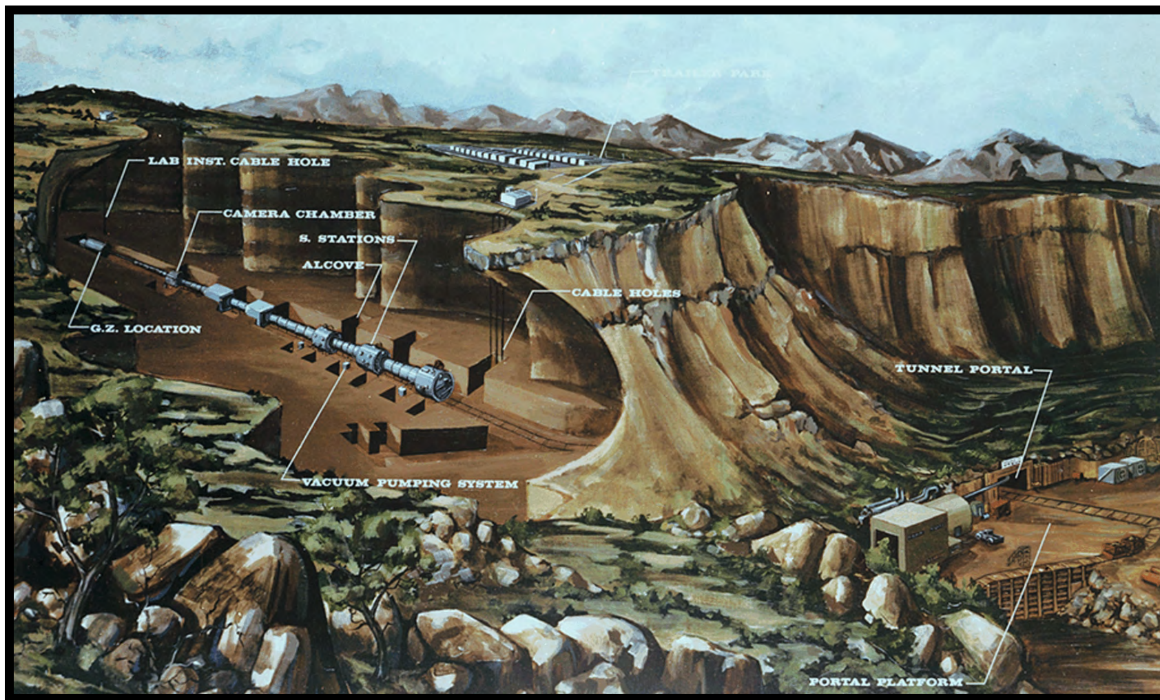
Figure 5. Typical layout of an underground nuclear weapons effects test (photograph NF-2054, on file at Remote Sensing Laboratory, Las Vegas, Nevada).
