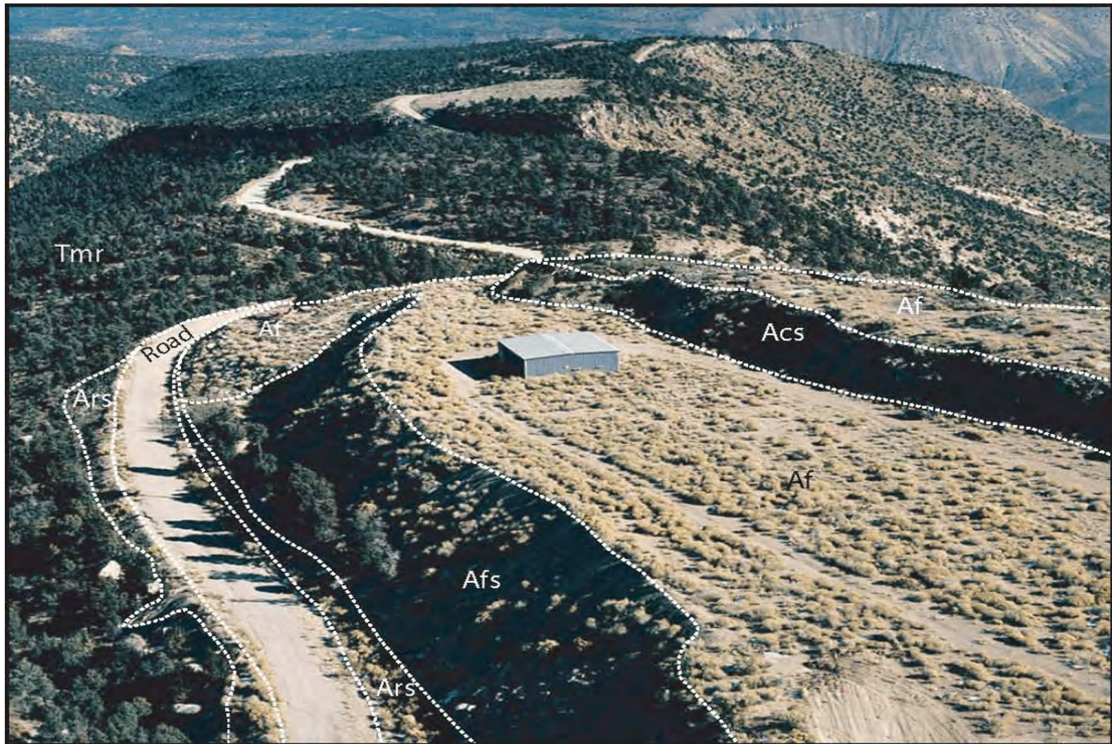
Figure 108. View north of the U12n Tunnel trailer park. Illustrated are cut slopes in the Rainier Mesa Member of the Timber Mountain Tuff (Acs), fill areas (Af), hillslopes adjacent to fill pads (Afs), and road side cast (Ars). Area denoted Tmr is the Rainier Mesa Member of the Timber Mountain Tuff and is generally covered by a thin mantle of colluvium. (modified from photograph NF-13505, on file at the Remote Sensing Laboratory, Las Vegas)
