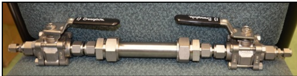
Figure 1. Sample holder for NO 2 aging of Ag 0 -functionalized aerogels.
