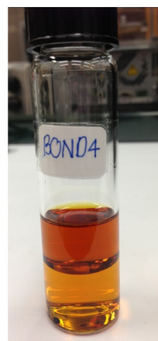
Figure 32. Polymerization of middle fraction during hydrodeoxygenation
