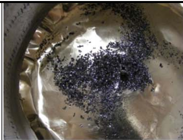
Graphite-on-Steel Test at 200°C (Test 9)
