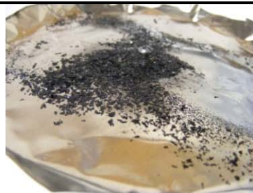
Graphite-on-Steel Test at 200°C (Test 9)
