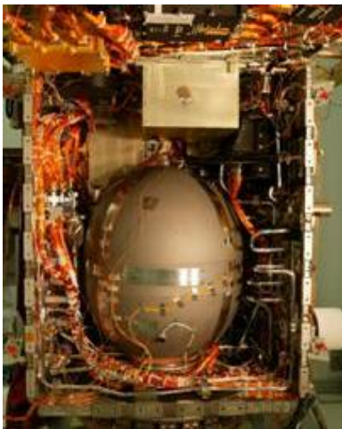
Figure 1. Electrical power and signal cables on a spacecraft.
