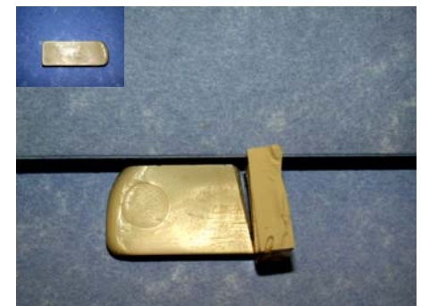
Short shot at 140°C, 100% speed, 50% pressure, 75% fill
