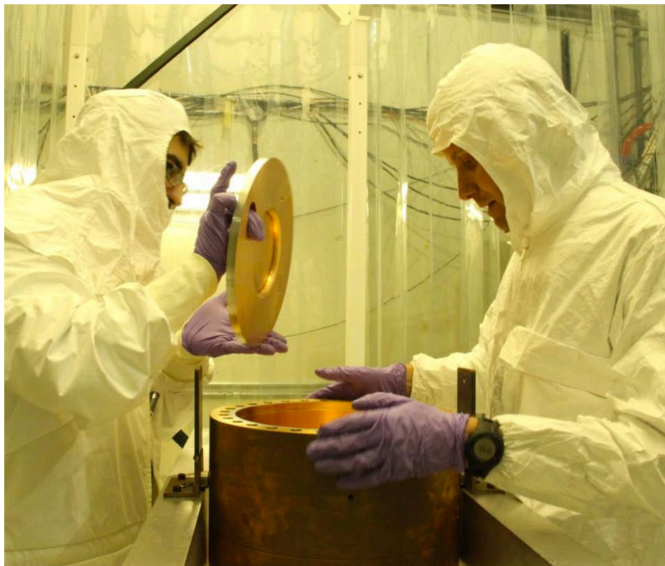
Figure 1: Gene Flanagan and Grigory Kazakevitch of Muons, Inc. showing the removable endplate of the All Seasons Cavity. The pillbox cavity, constructed to operate under vacuum or with up to 100 Atm of hydrogen gas, has so far only been used for vacuum tests. These have led to new insights for RF cavities operating in strong external magnetic fields. As a true pillbox cavity, it could be the first to operate under high pressure with the geometry expected in muon beam cooling channels.
