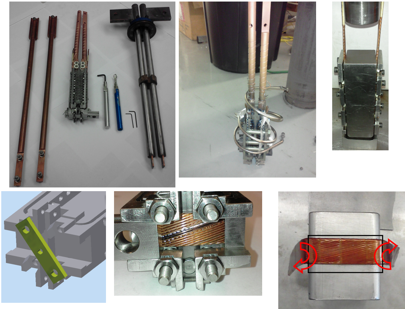
Figure 3.2.1. The \text{Nb}_3\text{Sn} Single-Strand Excitation ICR/Current-Sharing Probe.
