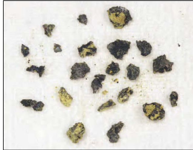
Smaller steel pieces recovered – mixed cover plate and ball materials
